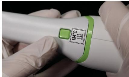
*Autoclave Tips have the autoclave symbol. See "Instructions for Autoclaveable Tips" on page 18.*
