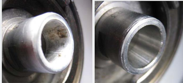
Clean the outside of the collets as well as the inside. Dirt on the outside (as shown on right) can also cause the tools to “walk” if the collet cannot clamp properly.
