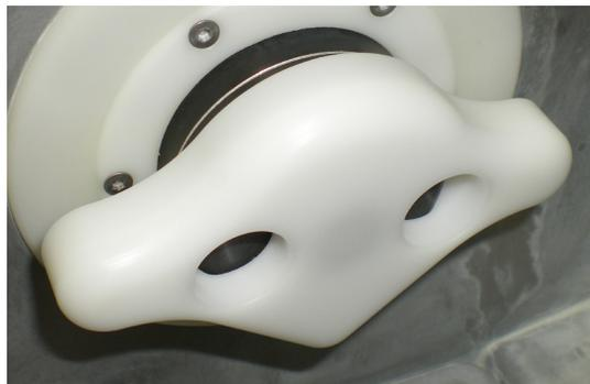
**Spindle Cap Tool in locked position -
