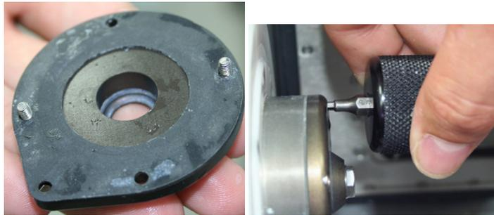
Tighten the screws with the hex wrench side of the collet tool. **Use your fingertips** to turn the tool to avoid using too much torque.
