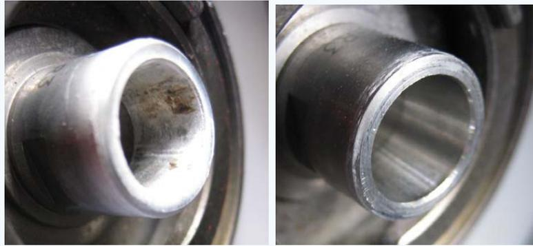
Clean the outside of the collets as well as the inside. Dirt on the outside (as shown on right) can also cause the tools to “walk” if the collet cannot clamp properly.
