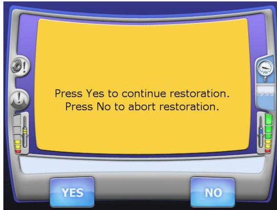
If the restoration has black marks or has come off of the mandrel, click No. The lid pops open. Remove the block. Select the job to restart milling. The system will prompt you to insert a new block at the beginning of the restarted milling process.
