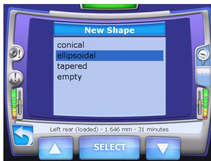
**5 Highlight the shape of the new tool or touch empty to remove the tool without a replacement.**
