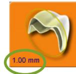
**Example A:** In the example below, the majority of the spacer follows the contours of the preparation (highlighted in green). There is a section of extra spacer where the tools had to overcompensate for the sharpness of the preparation (highlighted in orange).
