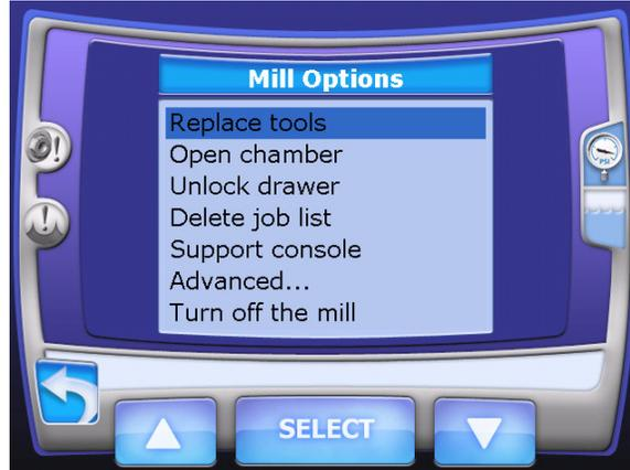
2 Highlight **Replace tools** by either touching the screen or using the up/down arrows and touch **Select**.
