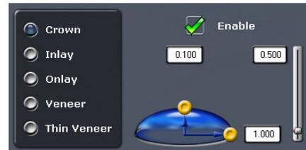
The effects of this tool are most easily seen on pre-op cases where there is a gap between the margin and the pre-op template, however this tool can be used on all cases to ensure sufficient material thickness and avoid chipping during milling.
